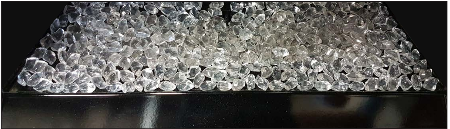
Figure 38. Glass Media Installation
