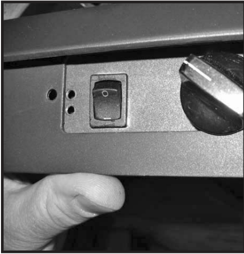
Figure 18: Reinstalling the Speed control assy.
