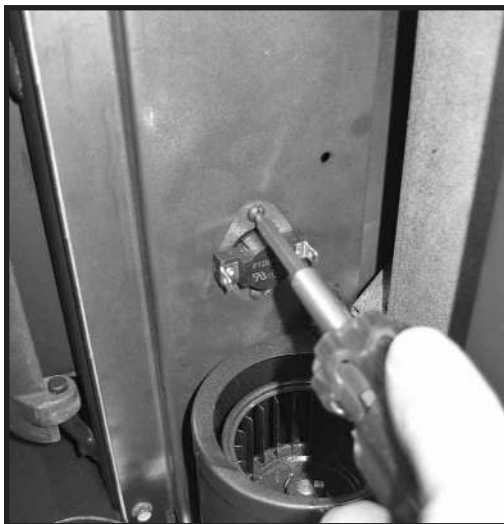
Figure 20: Removing thermal switch.
