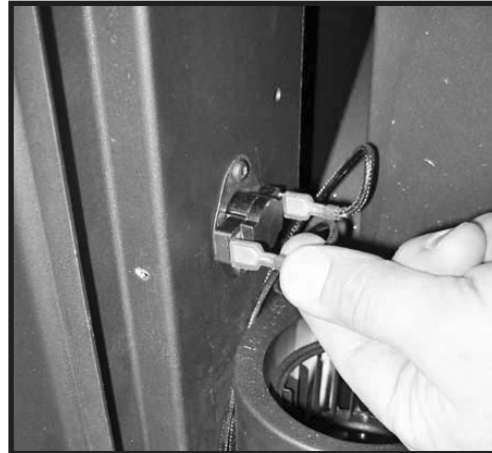
Figure 14: Disconnecting thermal switch.
