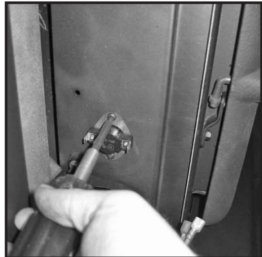
Figure 21: Relocating thermal switch to left side.
