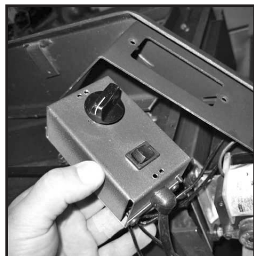
Figure 17: Removing speed control assembly.
