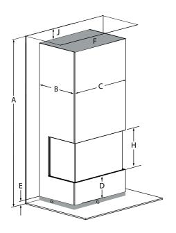
Top only heat release with front and sides intake
