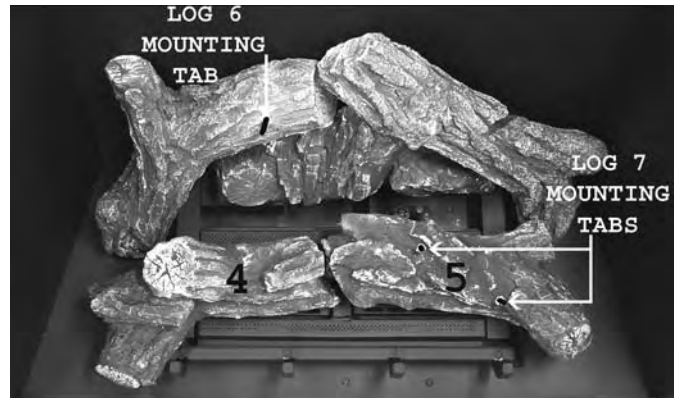
STEP 3: Locate 2 holes on the bottom of logs #4 and #5. Position them onto left and right log placement tabs.
