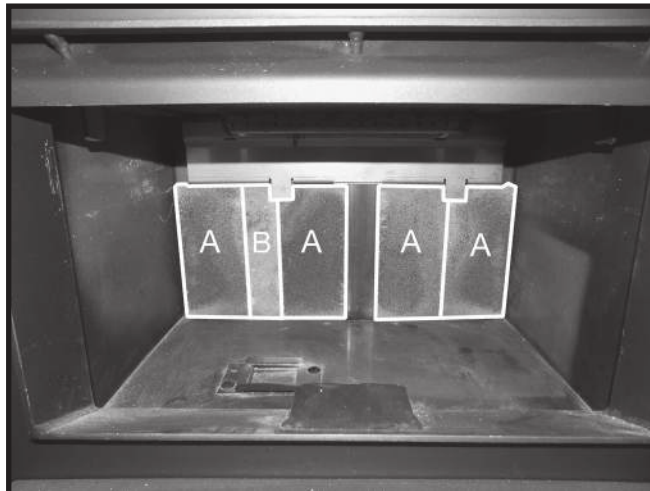
Figure 16: Left side rear wall A and B brick placement.
