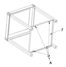
Slide the bottom shelf (7) into the corresponding position of each leg, with four M6\*12 screws (A) tighten by hand. (as shown)
