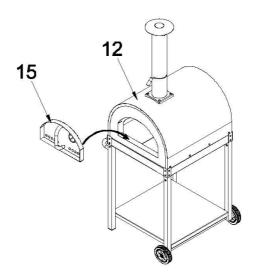
Slide the Door assembly (15) into the corresponding position (Front door opening) of the firebox assembly (12).
