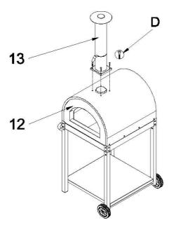
Place and fasten the Chimney assembly (13) onto firebox assembly (12) with four M6\*38 screws (C) tighten by hand.
