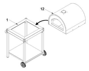
The Firebox assembly (12) is lifted and placed onto the corresponding position of the frame roof (1).
