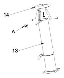
Affix the Chimney cover (14) onto the Chimney assembly (13) with three M6\*12 screws (A) tighten by hand.
