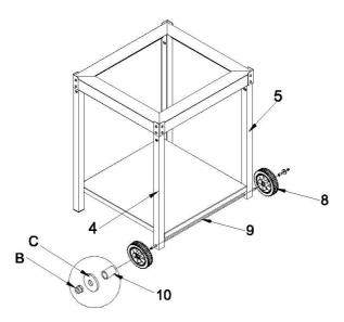
Slide the Axle (9) through the wheel legs (4 and 5), slide a Wheel (8) and Sleeve (10) and Flat washer (C) onto axle end, Thread two M6 lock nuts (B) onto each long end and tighten with a wrench. The wheel should spin, but not wobble.
