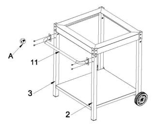
Slide the Side handle (11) onto Left front leg (2) and left back leg (3,) with four M6\*12 screws (A) tighten by hand.
