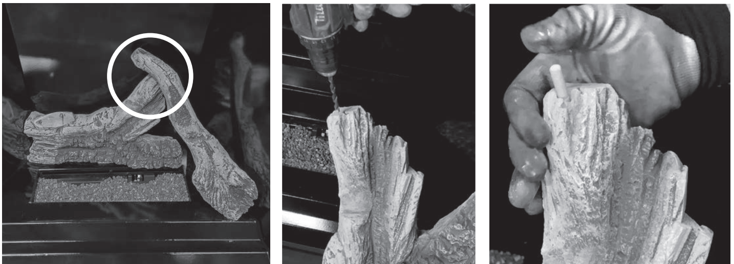
Figure 75: Using a 5/16 drill bit, drill a hole 1in deep in the rear log as shown above. Insert the log pin that was supplied with the unit into the hole.
