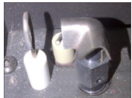
Figure 25: Correct Pilot Position
