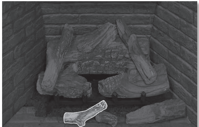
Figure 85: Log Set Installation - Step 8
