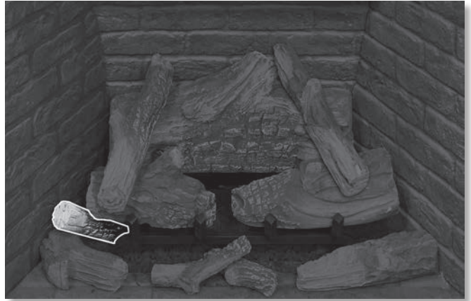
Figure 87: Log Set Installation - Step 10
