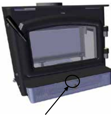
Primary Air Damper Left - Open Right - Closed
